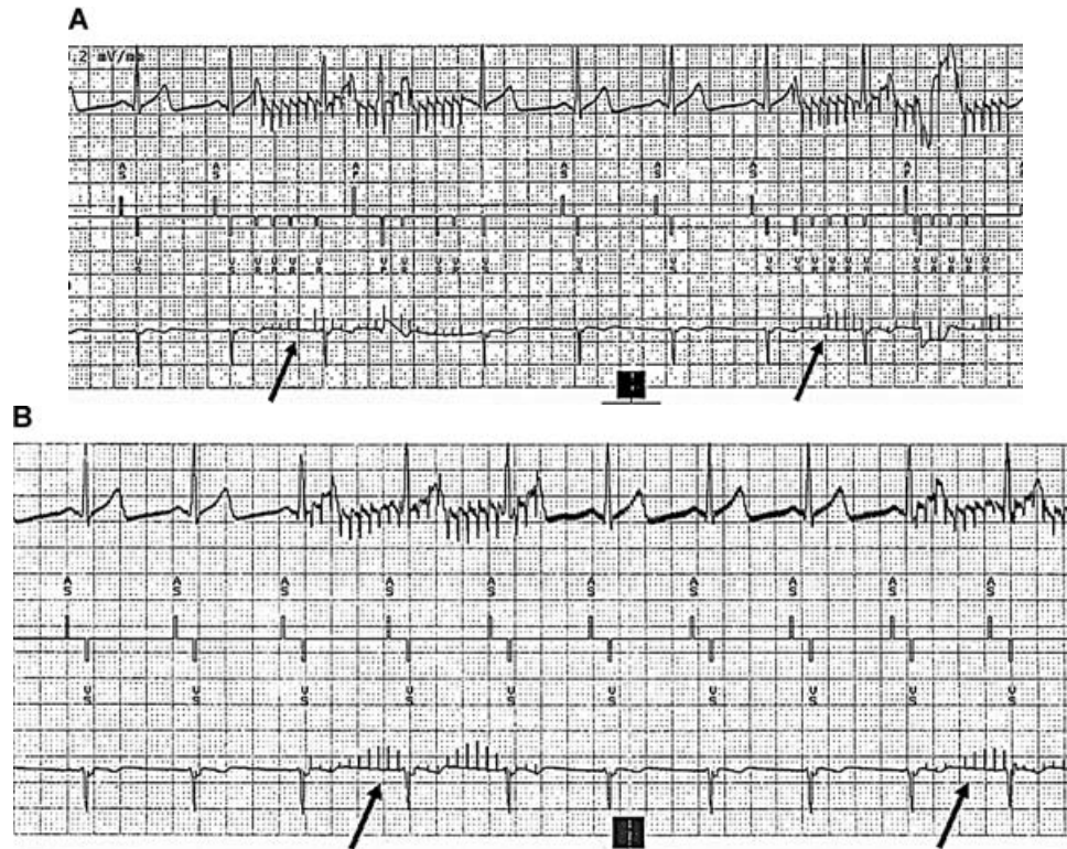
Figure 2. (A and B) Top line shows the surface ECG, middle-line marker annotations of the cardiac pacemaker (AP = atrial pacing; AS = atrial sensed event; VP = ventricular pacing; VR = ventricular event within refractory period; VS = ventricular sensed event), and the bottom line the bipolar ventricular electrogram. On panel 2a, the ventricular sensitivity of the pacemaker is set at 1.0 mV and pacing artifacts (arrows) of the diaphragm pacemaker are sensed by the cardiac pacemaker (see annotations in marker channel). After reducing the ventricular sensitivity (Panel 2b), the pacing artifacts of the diaphragm pacemaker are no longer sensed by the cardiac pacemaker.
